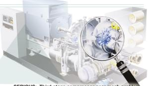
SERIOUS: Third-stage compressor gear mesh problem MODERATE: Third stage compressor bearing wear
