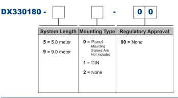
Example Part Number: DX330180-91-00 9 meter system length, DIN mount
